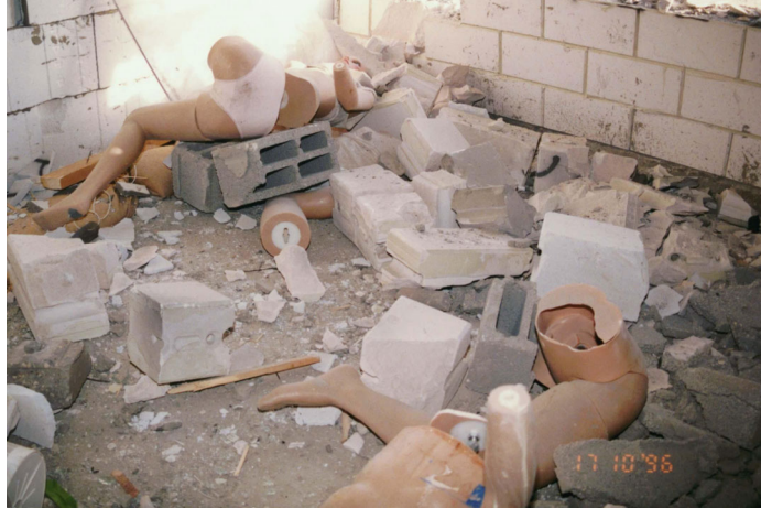
Figure 30: CMU Debris Impact on Mannequins
