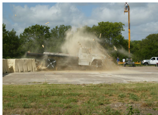
Sand-filled Plastic Barriers
