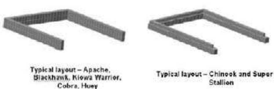
Figure 8-21. Typical revetment configurations for Army helicopters
