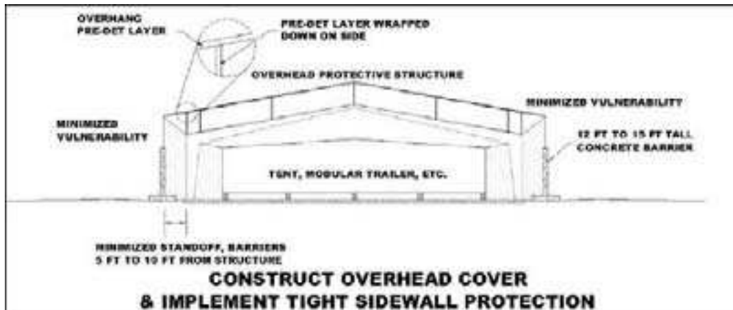
Figure 8-33. External protection, overhead cover and tight sidewall protection
