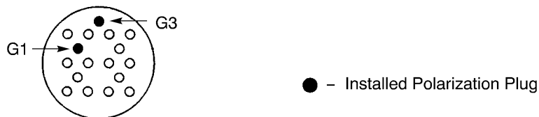
10-60540-2 RELAY SOCKET POLARIZATION - KEY G2 Figure 7
