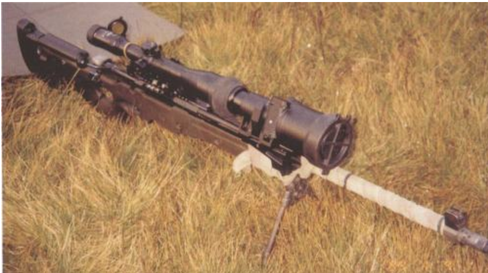
The German Army night optical sight unit fitted to the G22. Note the rubber interface between the sight and the telescopic sight objective lens to form a light-proof seal between the two units.
