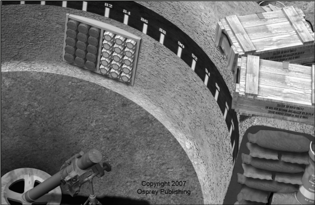
Figure 3-1. Mortar pit with mil markings
