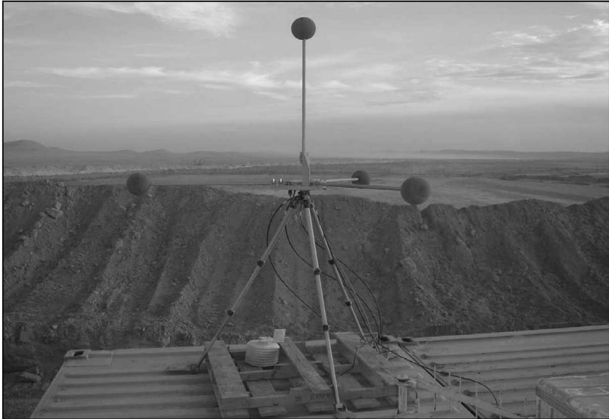
Figure 4-2. Unattended transient acoustic measurement and signature intelligence system
