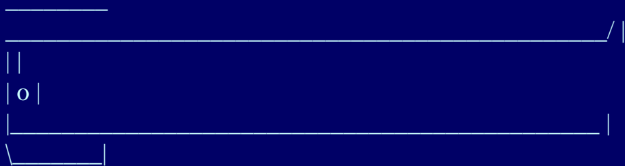
fig. 1 pipe with one end flattened and fuse hole drilled (top view)
