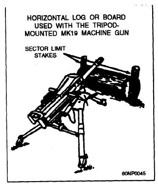
Figure 4-30.—Aiming stakes used with a log.
