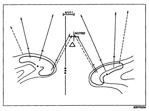
Figure 4-13.—Coverage for a gap.
