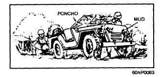
Figure 5-4.—Cover portions of vehicles that reflect light.
