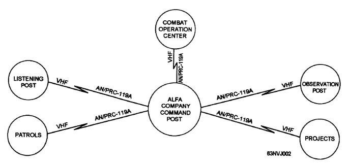
Figure 2-2.—Company CP radio plan.
