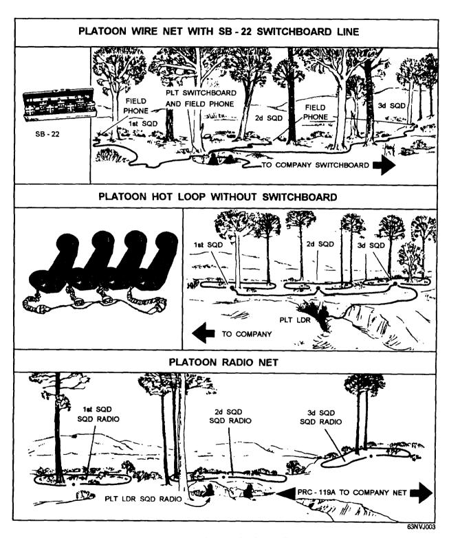
Figure 2-3.—Various platoon and radio net illustration.
