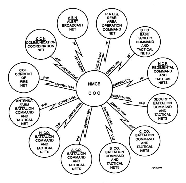
Figure 1-10.—COC radio plan.
