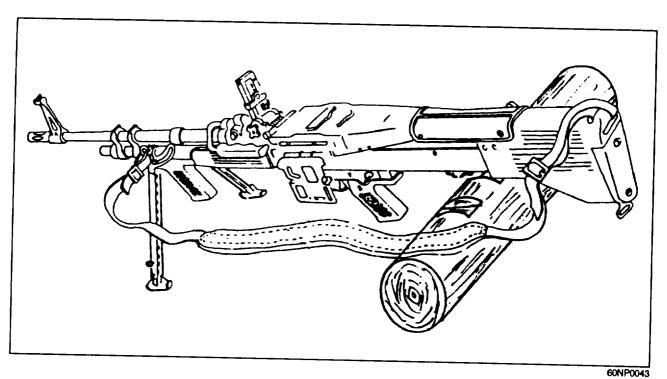
Figure 4-28.—Notched log under receiver.
