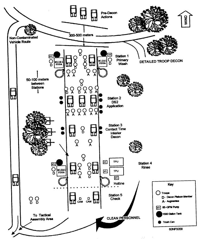
Figure 6-8.—Optimum DED for an M12A1 PDDA-equipped layout.
