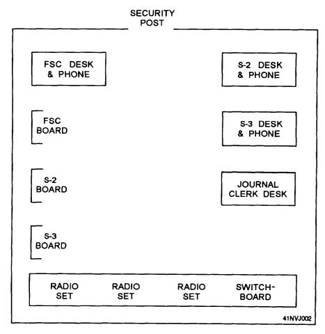
Figure 1-8.—Internal arrangement of COC.
