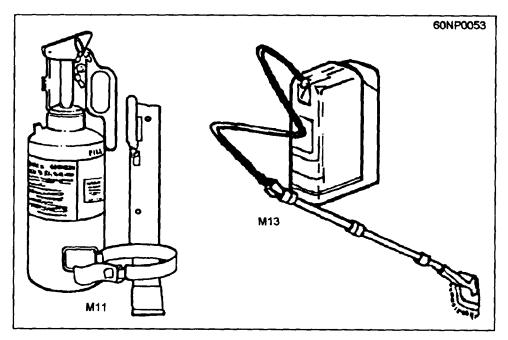
Figure 6-3.—Portable decon apparatus.
