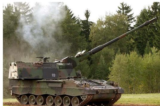
From a firing position within the camp perimeter, the Armoured Howitzer 2000 is capable of supporting own forces within a radius of 30 kilometres. The weapon system is responsive, precise and combat serviceable in any weather conditions. Combined with the COBRA system, hostile artillery and mortar positions can be engaged quickly and effectively.
