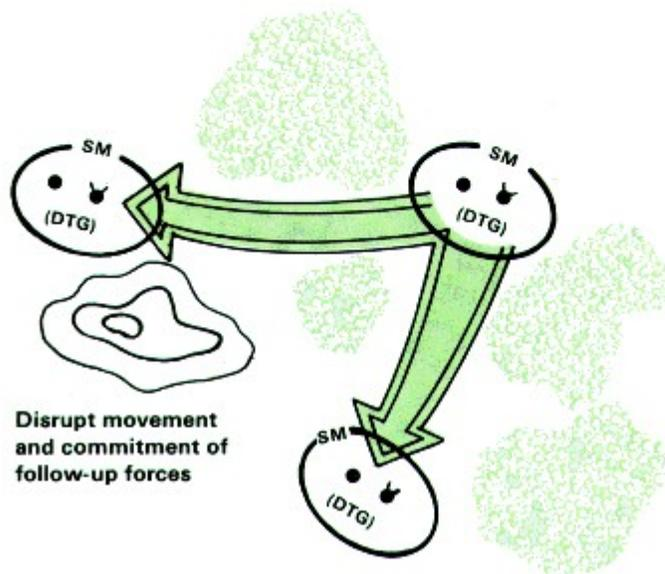
Mines are used extensively where the existing obstacle structure is weak or nonexistent. They should also be used with other reinforcing obstacles, such as tank ditches, to make breaching and clearing more costly and time-consuming to the enemy.
