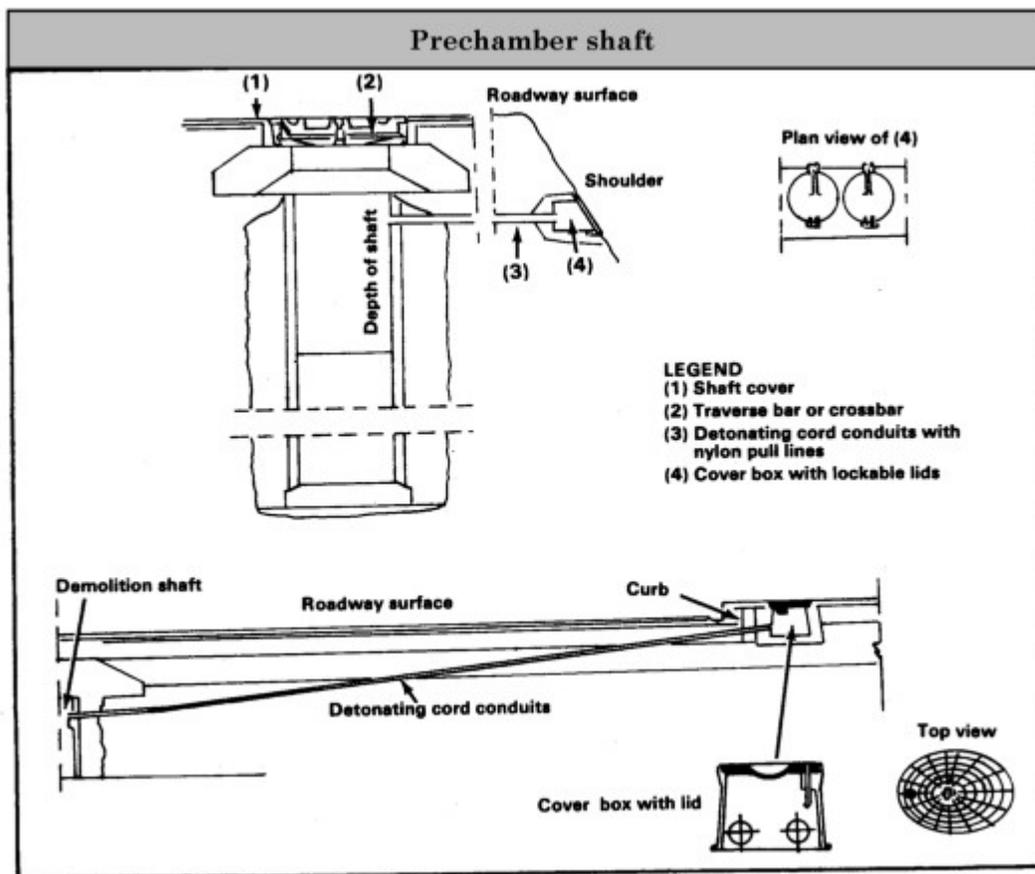
The demolition material required for a prechamber shaft system is stored in a nearby 5-ton bunker complex and is earmarked for the sole use at its designated obstacle site. The prestocked demolition material consists of:
