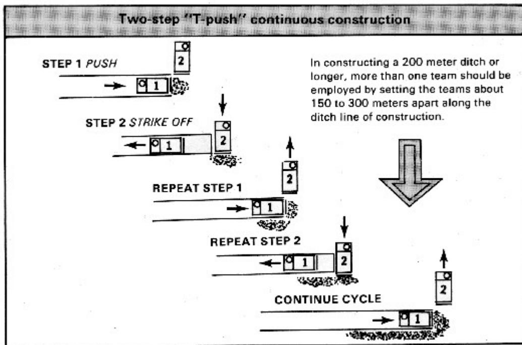
**One dozer and one scoop loader, grader, or CEV as a team.** This step is performed the same as the previous method except that the loader or CEV is used in place of vehicle #2. The grader is available to keep the berm straight and built up. After the ditch is constructed, and if time permits, the berm can then be further shaped. Normally, this method would be less productive than the first method. Again, more than one team may be used to construct the ditch.
