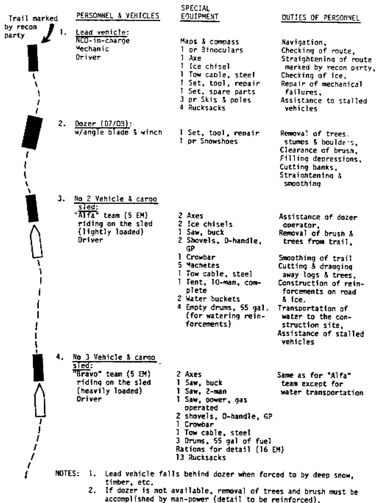
Figure 5-6. Construction detail for winter roads.
