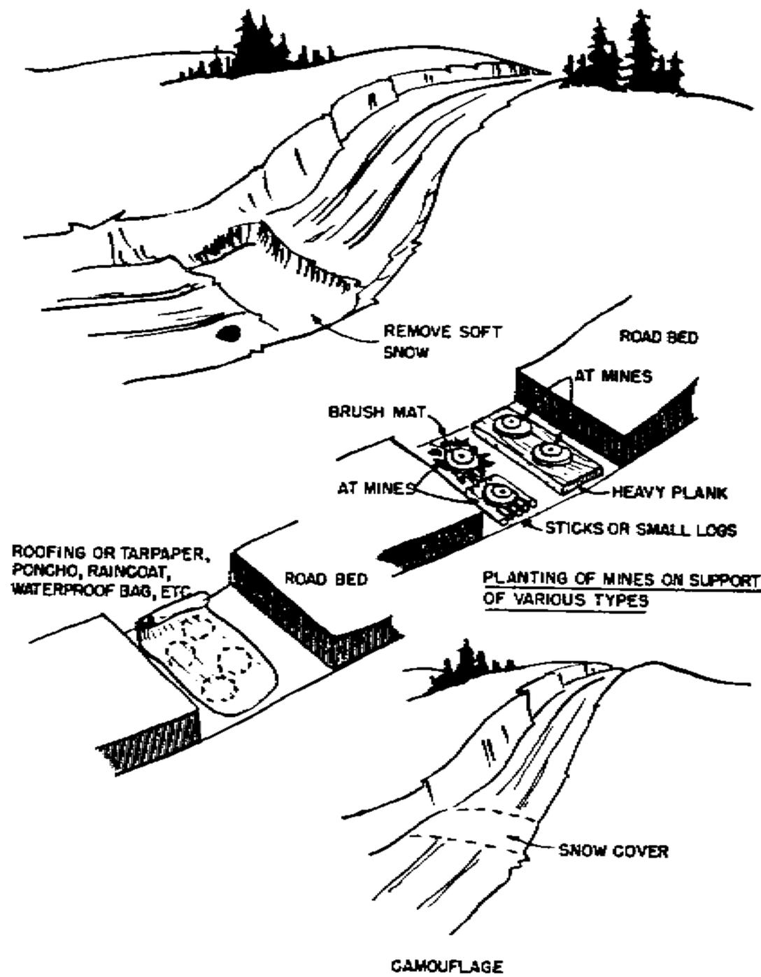
Figure 6-32. Laying mines in deep snow.
