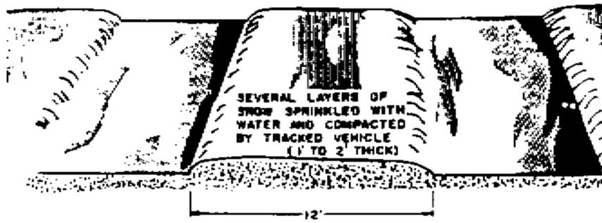
Figure 5-7. Road reinforced with snow.
