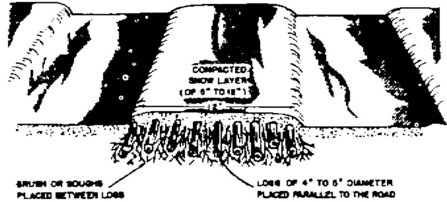
Figure 5-9. Road reinforced with brush, logs, and snow.
