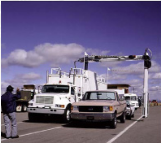
Figure 1: Mobile VACIS - Gamma Ray Imaging System
