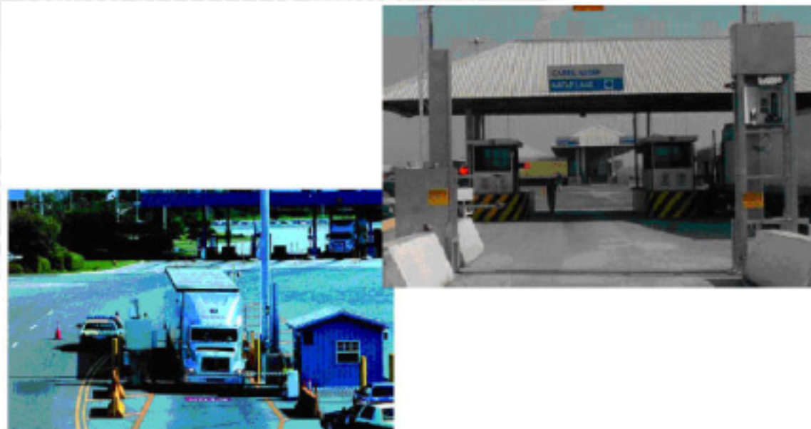
Top: Figure 5: Fixed / Portable Vehicle X-ray Inspection Systems (Imaging)
